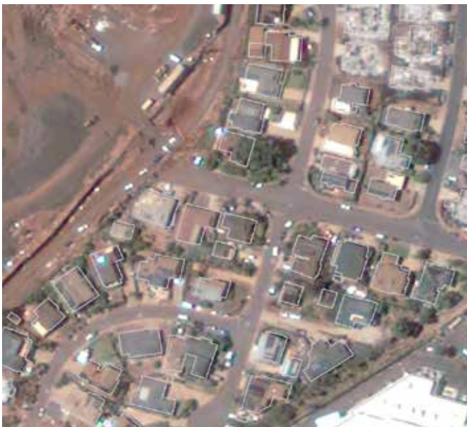
Building Footprint Feature Extraction
